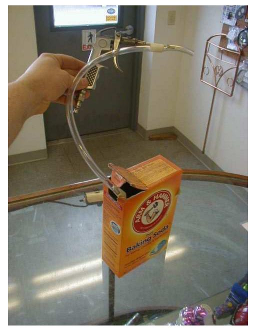
WARNING: Blasting should ONLY be done outside in a well ventilated area such as a patio or concrete driveway. Of course proper eye protection and a face mask should always be worn. Baking soda is not poisonous but it feels like your breathing a soft drink if you inhale it and it's irritating, so protect those lungs!!
