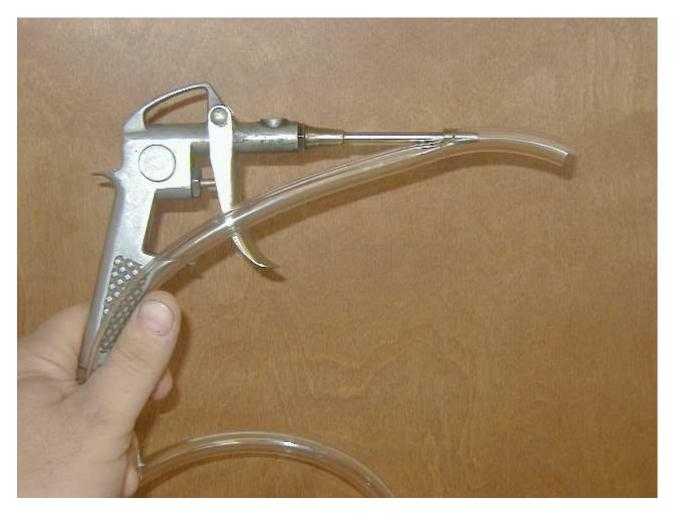
Positioning your wand tip like this will create a ventricle effect in the hose causing the soda to be pulled up from the box and mixed with the high pressure air from the wand. Use one length of tape to wrap around the end of the air wand and hose. This will keep the hose in the proper position on the wand tip during blasting.
