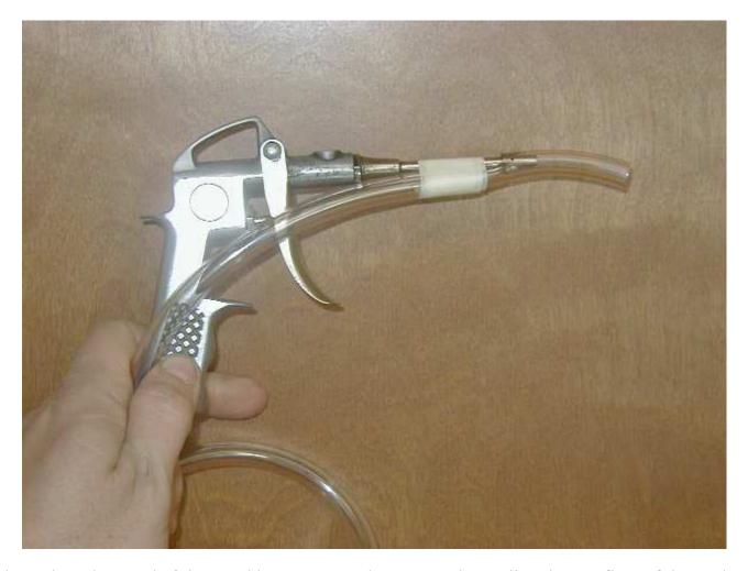
I cut the other end of the vinyl hose at a 45 degree angle to allow better flow of the soda into the hose. Then I tape the piece of dowel, metal rod or wire to the other end of the hose. This will help keep it from curling up in the box of soda and help you keep good flow into the hose.
