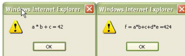
Figure 13-13: Two watchpoints revealing logic error — concatenation instead of addition
