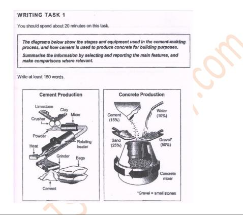
The diagrams highlight the steps involved in producing cement and the process by which concrete is produced using cement.
