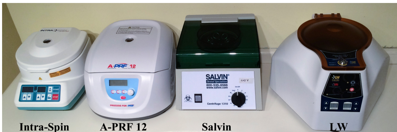
Figure 1. The 4 centrifuges used to produce L-PRF clots and tested in this study. From left to right: original L-PRF centrifuge (Intra-Spin, Intra-Lock), A-PRF 12 (Advanced PRF, Process), Salvin 1310 (Salvin Dental) and LW - UPD8 (LW Scientific).
