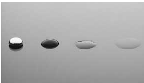
■ Figure 13-25 The cohesive forces are strongest in mercury and weakest in acetone. The stronger the cohesive force, the more spherical the drop will be.
