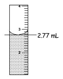
so that the line at the bottom of the meniscus gives the most accurate reading. In order to read any graduated cylinder accurately, it must be level (sitting on the counter, **NOT** hand-held). Your eye must also be perpendicular to the water level. Note that the graduations on all cylinders rise from the bottom up. That is, they indicate the volume **contained** in the cylinder.
