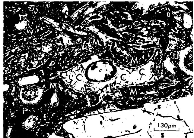
Figure 5. Photomicrograph of mordenite-rich tuff (sample G1-2291.1) from Bullfrog Member of the Crater Flat Tuff in drill hole USW-G1, showing well-preserved vitroclastic texture. Pseudomorphs of original vitric materials are defined by a layer of compact fibers of mordenite (M). Large pseudomorph in the central part of the photo shows relatively large, blocky crystals of clinoptilolite (C) that grew on a thin layer of compact fibers of mordenite.
