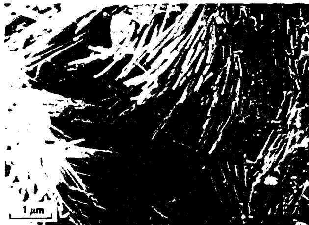
Figure 9. Scanning electron micrograph of sample UE25-2900.4 from the tuffaceous beds of Calico Hills in drill hole UE25b-1H, showing compact layer of filiform mordenite that projects into the hollow interior of a pseudomorph of a shard.
