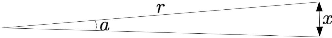
Astronomers use geometry to measure the sizes and distances of planets and nearby stars. If we can draw a triangle like the one above then there's a geometric relationship between size  $x$ , distance  $r$  and angle  $a$ :
