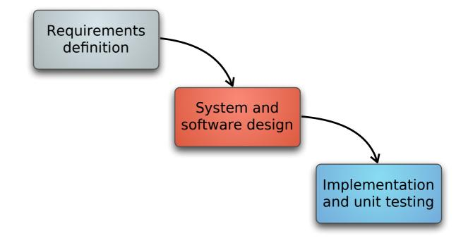
Software Process Models - The Waterfall Model 9 4. Integration and system testing Program units are integrated and Requirements definition tested as a complete system. System and software design Implementation and unit testing
