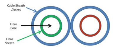
Typical Cable Construction – Multi-Core Cable
