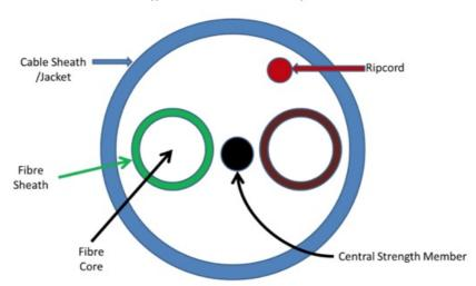
Typical Cable Construction - TwinFlex
