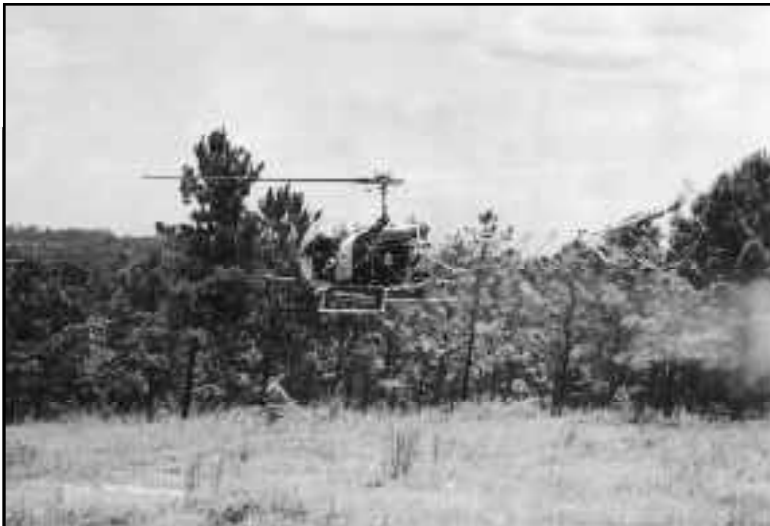
H-13 helicopter armed with two .50 ANM machine guns and two 6-tube 2.75-inch Folding-Fin Aerial Rocket clusters. Matteson Range at Fort Rucker, AL October 1958
