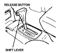
The shift lever has seven positions. It must be in Park or Neutral to start the engine. When you are stopped in D4, D3, 2,1 or R, press firmly on the brake pedal and keep your foot off the accelerator pedal.
