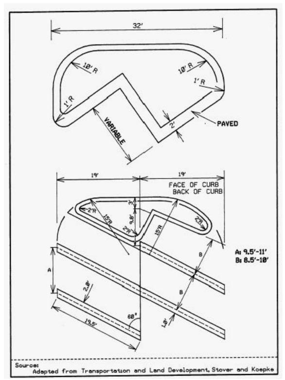
Figure 9-5 Typical End Island Designs (60 Degree Parking)
