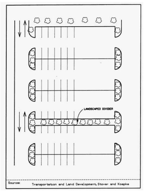
Figure 9-3 Planted Strips to Prevent High Speed Diagonal Movements
