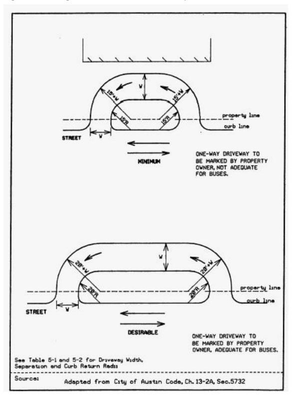
Figure 9-8 Design Criteria for Semicircular Drop-offs
