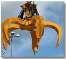
unique hydraulic self lubrication system uses the grab's working pressure to drive the self-lubrication grease pump. The system pressurizes grease up to 250 bar and injects grease to all main bearing and cylinder bearings —15 bearings in total.
