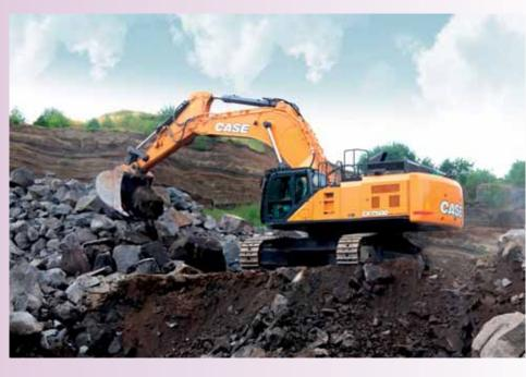
for greater power and productivity, and arm and bucket cylinders are larger to help improve performance. And the machine can be operated in one of three operating modes — Automatic, Heavy and Speed Priority — to provide the optimal and most efficient use of hydraulic and engine power.
