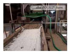
With some dust-prone products it is not appropriate to use water, as this may affect the product quality or cause damaged to processing.
