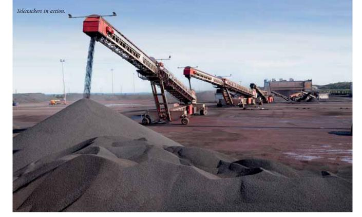
equipped with two hoppers, one for feeding with a wheel loader and one with dump trucks. These units can also be connected together to move the material from the train unloading facility directly under the crane, avoiding the processing phase. The conveyor system is also suitable for different type of solid bulk cargo.
