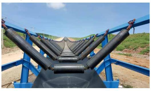
systems; there is a considerable advantage in terms of energy consumption due to the considerably smaller pushing rolling resistance. With a belt width of 2,000mm and a belt length of 1,887m, a reduction in the pushing rolling resistance of up to 300kW is achieved. Taking into account the fact that the energy is generated in a coalfired power plant, this means a CO<sub>2</sub> saving of approximately 2,400 tonnes per year.
