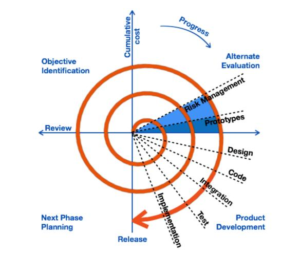
This model considers risk, which often goes un-noticed by most other models. The model starts with determining objectives and constraints of the software at the start of one iteration. Next phase is of prototyping the software. This includes risk analysis. Then one standard SDLC model is used to build the software. In the fourth phase of the plan of next iteration is prepared.
