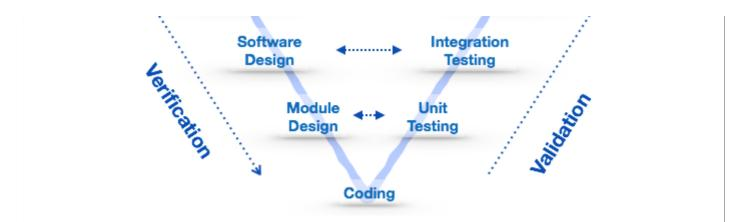
At every stage, test plans and test cases are created to verify and validate the product according to the requirement of that stage. For example, in requirement gathering stage the test team prepares all the test cases in correspondence to the requirements. Later, when the product is developed and is ready for testing, test cases of this stage verify the software against its validity towards requirements at this stage.
