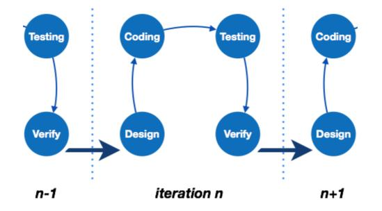
The software is first developed on very small scale and all the steps are followed which are taken into consideration. Then, on every next iteration, more features and modules are designed, coded, tested and added to the software. Every cycle produces a software, which is complete in itself and has more features and capabilities than that of the previous one.
