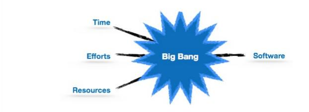
For this model, very small amount of planning is required. It does not follow any process, or at times the customer is not sure about the requirements and future needs. So the input requirements are arbitrary.
