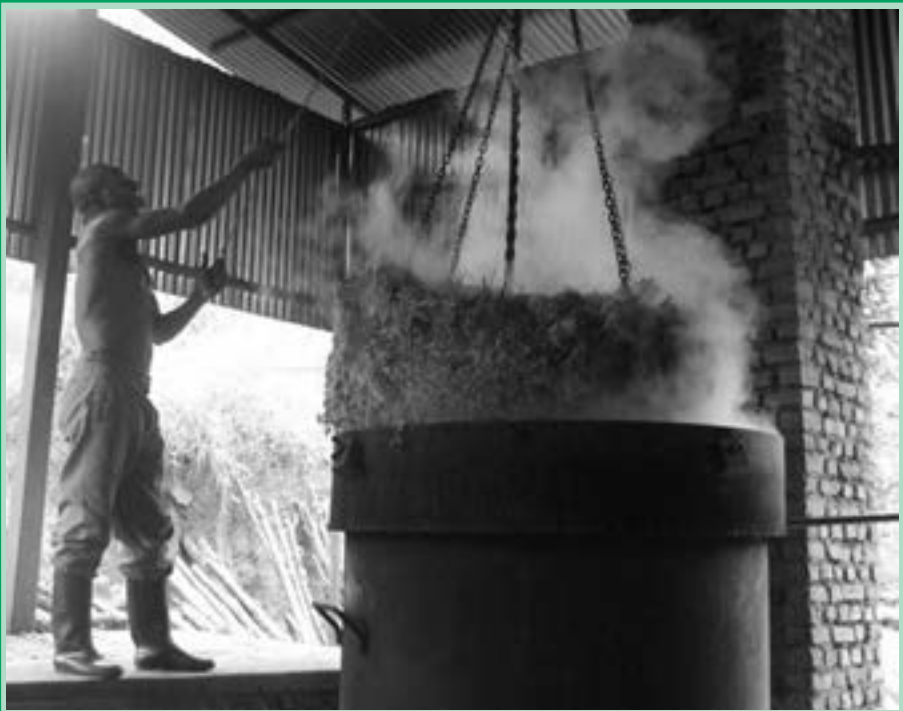
FIGURE 22 Removing geranium material from a small still following steam distillation of essential oil
