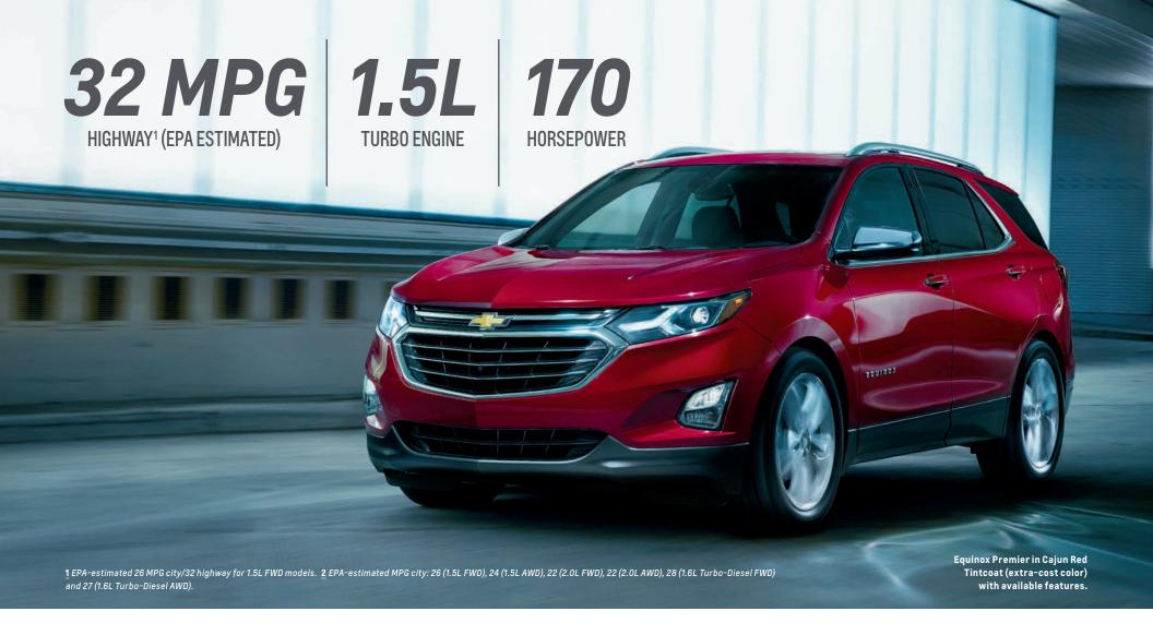
1.5L TURBO ENGINE. This new turbocharged 4-cylinder engine uses the technologies of Continuously Variable Valve Timing and Direct Injection to deliver responsive performance with unexpected efficiency. It puts 170 horsepower at your command, along with 203 lb.-ft. of torque. EPA-estimated fuel economy is 26 MPG city/32 highway (FWD) and 24 MPG city/30 highway (AWD).
