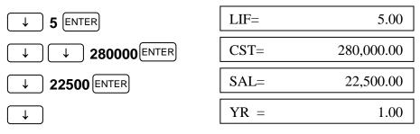
3. Display the first year depreciation data. At this point, the calculator has already calculated this data for the first year. The remaining steps cause the values to be displayed.
