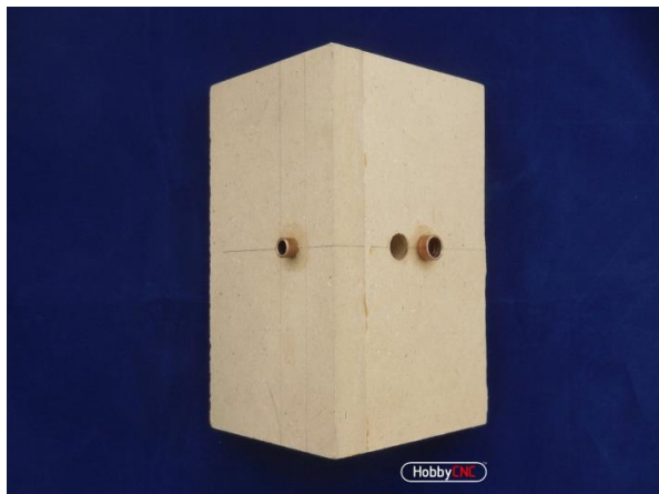
Figure 14 – Cross Dowel Jig, top view
