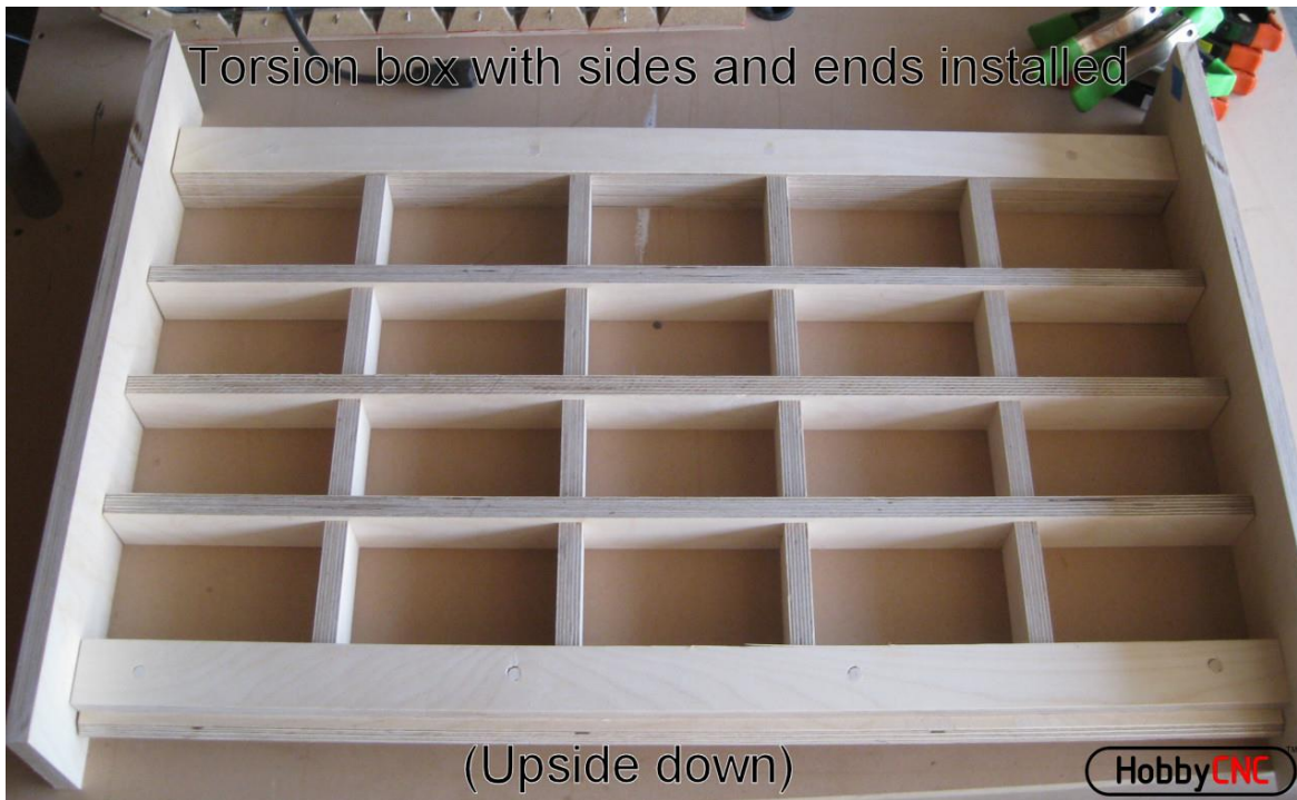
Figure 11 - Underside of my Torsion Base (as built)
