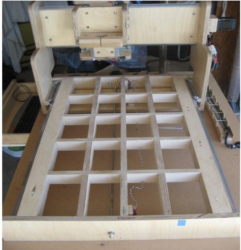
Figure 12 - Torsion Base (without top) test X-Axis gantry
