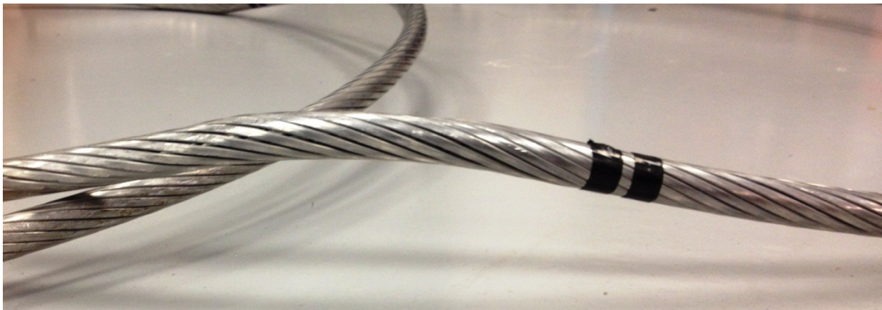
Figure 6: If the conductor has taken a “set” from bending, the bent section should be cut out and a full tension splice installed. The section shown was bent 90° around a six (6) inch radius. The tensile test showed a 25% strength reduction.
