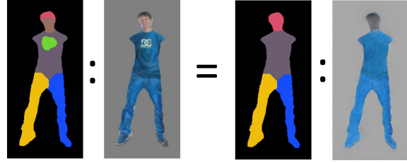
Figure 4: Synthesizing back texture. We transform the back texture construction into a texture-by-numbers problem. We first modify the body label map by labeling undesired region with different colors (i.e., face and shirt logo) to create the source label map. In this example, we then use the original body label map as the target label map for the back; thus, the constrained texture synthesis will not use pixels covered by the new labels when creating the back texture, so that the face and logo do not appear on the back.
