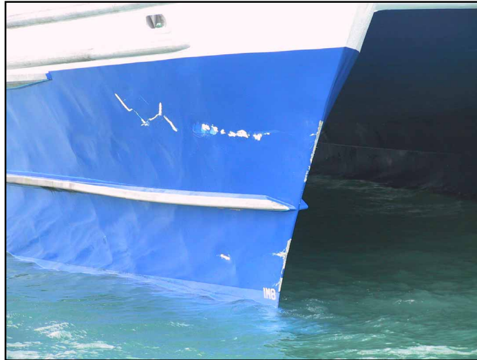
Figure 6 Damage to the Quickcat 's hull
