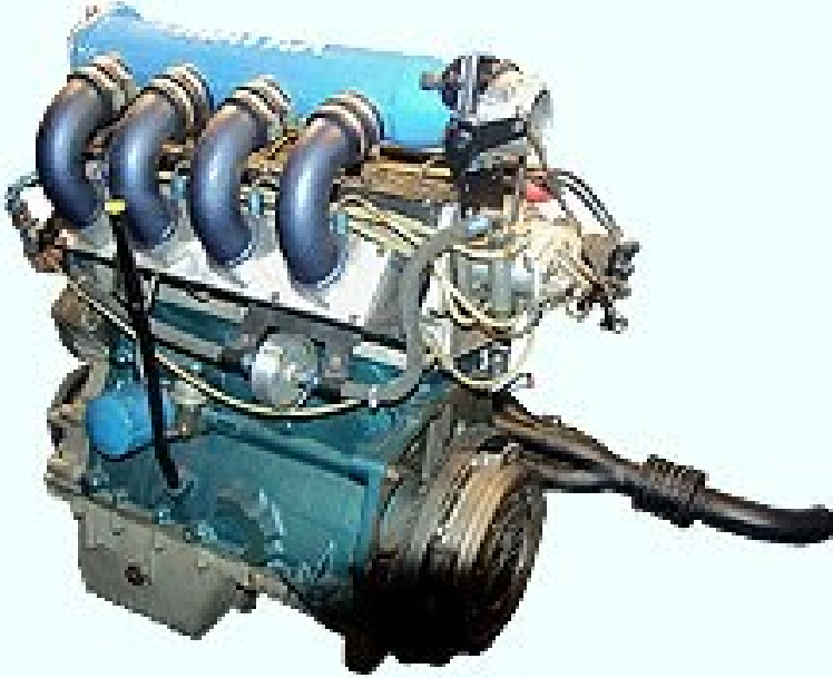
4S engine: 175.5 bhp @ 6.000rpm with 85% Torque at 2500rpm
