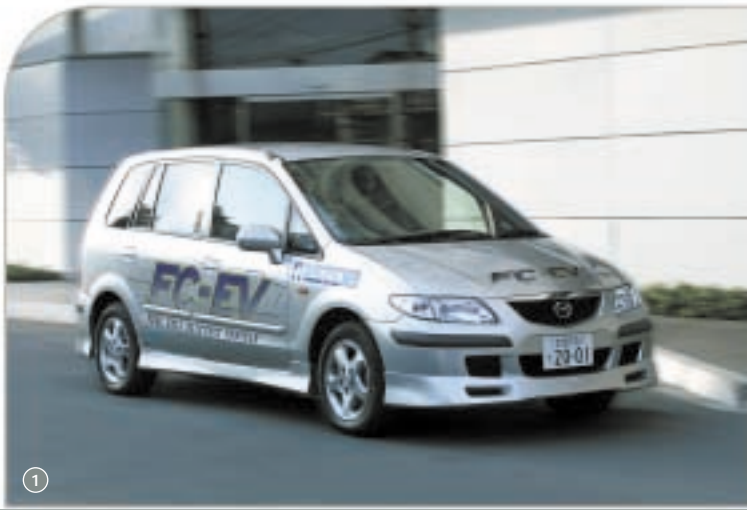
① ② Mazda has developed the Premacy FC-EV, a new fuel cell electric prototype that will be used for Japan's first test run of fuel cell vehicles on public roads with the support of the Ministry of Economy, Trade and Industry. Using the Premacy FC-EV, Mazda is participating in a joint project with DaimlerChrysler Japan Holding, Ltd. and Nippon Mitsubishi Oil Co.
