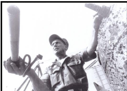
Nha Be Vietnam, 1966: LCDR Talarico holding detonator/booster assembly of captured and safed Russian MKB chemical horn mine. (photo courtesy Navy and Marine Corps EOD Association)
