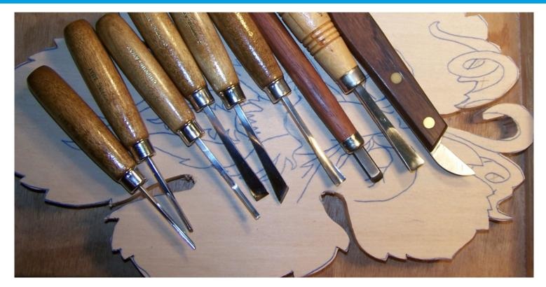
From left to right - u-gouge, micro v-gouge, v-gouge, straight chisel, skew chisel, large round gouge, bull nose chisel, wide sweep gouge, bench knife.
