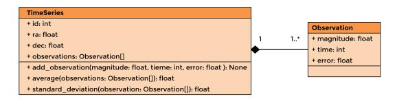
Figure 1.5: Example of the *composition* relation between classes in a UML diagram.
