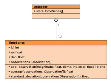
Figure 1.6: Example of the *agreggation* relation between classes in a UML diagram.
