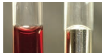
FIGURE 2.3 The water's surface (left, dyed red) is curved down because water has greater adhesion than cohesion. The surface of the mercury (right) is curved up because mercury has greater cohesion than adhesion.
