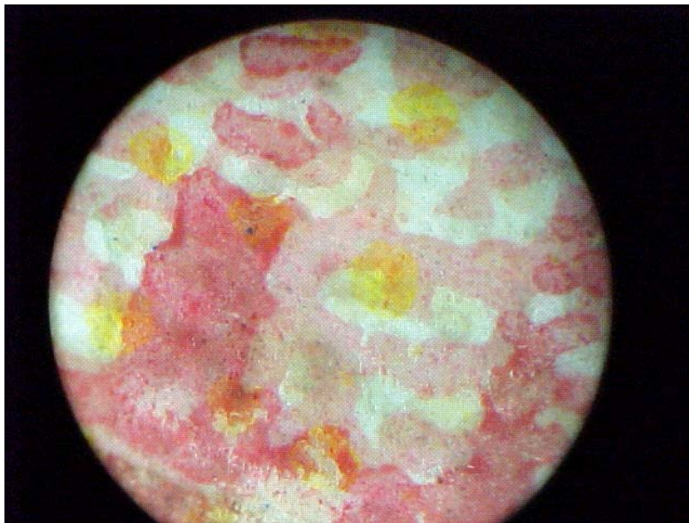
Chromolithography on an 1892 Trade card at 100X power. The ink is watery and messy, like a watercolor painting. No confusing this for a modern halftone print.
