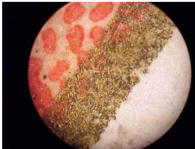
Vintage gilding. Microscopic view (100X Power) of the gilding on a turn of the century card, with the flakes of tarnished metal.
