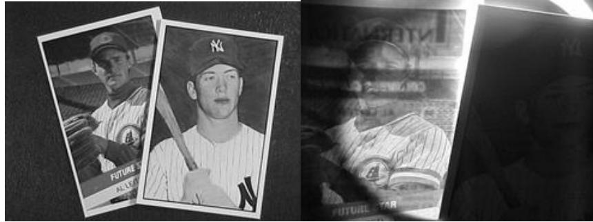
While the two 1980s cards on the left appear to be made of the same card stock, when put in front of a light the opacities are quite different.
