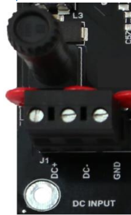
FTS 371 FTC SMART DC Input Power Connections
