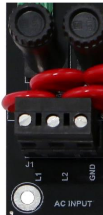
FTS 371 FTC SMART AC Input Power Connections
