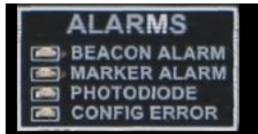
Alarm Indication LED's
