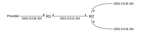
Interface 0 of R1 would be assigned an address from the /64 block 2001:0:0:0/64, perhaps 2001::2.
