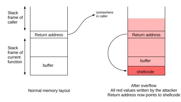
The right side shows the result after the attacker has written shellcode to the buffer, and, by overflow, has also overwritten the return\_address field on the stack so that it now points to the shellcode. When the function exits, control will be passed to the code at return\_address, that is, to the shellcode rather than to the original caller. The shellcode is here shown below return\_address in memory, but it can also be above it.
