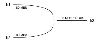
We want the r-h3 link to be the bottleneck, making this an instance of the singlebell topology (20.2.3 *Example 3: competition and queue utilization*). To do this, we need to be able to control the bandwidth, delay and queue size on the r-h3 link. (While this topology is fairly standard for TCP competitions, we really
