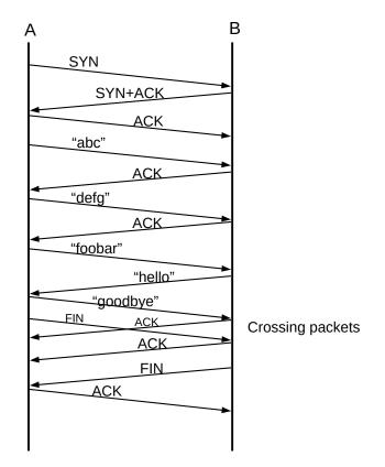
In terms of the sequence and acknowledgment numbers, SYNs count as 1 byte, as do FINs. Thus, the SYN counts as sequence number 0, and the first byte of data (the "a" of "abc") counts as sequence number 1. Similarly, the ack=21 sent by the B side is the acknowledgment of "goodbye", while the ack=22 is the
