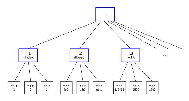
In all three tables here, the index columns are part of the table data. This is unnecessary; all the index columns are of necessity encoded in the full OID of any table entry. In SNMPv2 it is required (though not necessarily enforced) to in effect omit the index columns from the table as presented by the agent (though they are still declared); see 27.1.4 SNMPv2 Indexes.
