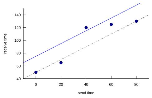
The diagram above plots the points of the table. The dashed line represents the expected arrival time for the corresponding send time; packets are late by the amount they are above this line. The solid blue line represents a playback buffer corresponding to 25 ms; packets arriving at points above the line are lost. The higher the line, the more playback delay, but also the more that playback can accommodate late packets
