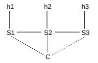
As with exercise 5.0, assume that the switches report packets to C only if they do not already have a forwarding-table entry for the packet's destination. After each report, C installs a forwarding-table entry on the reporting switch for reaching the packet's source address via the arrival port. At that point the switch floods the packet (as the destination must not have been known). If a switch can forward a packet without reporting to C, no new forwarding entries are installed.
