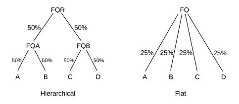
If all four input classes A,B,C,D are active in the hierarchical structure, then each gets 25% of the total bandwidth, just as for a flat four-input-class fair queuing structure. However, consider what happens when only A, B and C are active, and D is idle. In the flat model, A, B and C each get 33%. In the hierarchical model, however, as long as FQA and FQB are both active then each gets 50%, meaning that A and B split FQA's allocation and receive 25% each, while C gets 50%.
