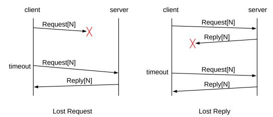
When the server creates reply[N] and sends it to the client, it must also keep a cached copy of the reply, until
