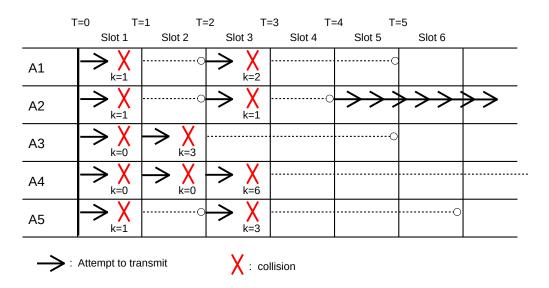
Fig. 11:: Ethernet collisions with exponential backoff
