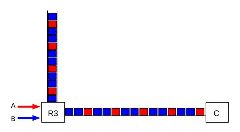
In the steady state here, A and B will use four and eight packets, respectively, of R3's queue capacity. As acknowledgments return, each sender will replenish the queue accordingly. However, it is not in A's long-term interest to settle for a queue utilization at R3 of four packets; A may want to take steps that will lead in this setting to a gradual increase of its queue share.
