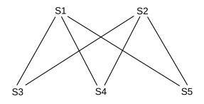
(a). $\Diamond$  Give network of surviving links after application of the spanning-tree algorithm. Assume the ID of switch Sn is n. In this network, what is the path of traffic from S2 to S5?
