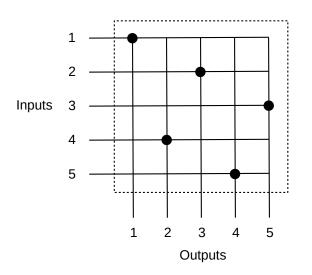
Fig. 17::  $5 \times 5$  crossbar with 5 parallel connections  $1 \rightarrow 1, 2 \rightarrow 3, 3 \rightarrow 5, 4 \rightarrow 2, 5 \rightarrow 4$
