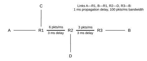
7.0. Suppose we have the network layout of the previous exercise, 6.0. Suppose also that the A–B and C–D connections have settled upon window sizes as in 6.0(b), so that each contributes 30 packets to R1's queue. Each connection thus has 50% of the R1–R2 bandwidth and there is no queue at R2.
