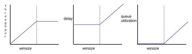
Graphs of winsize versus throughput, delay and queue utilization. Vertical dashed line represents winsize = bandwidth x no-load delay
