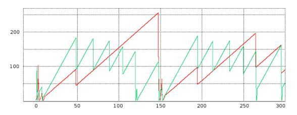
Here we have (without the queue data) a good example of highly **un**synchronized teeth: the green graph has 12 teeth, after the start, while the red graph has five. But note that the red-graph loss events are a subset of the green loss events.
