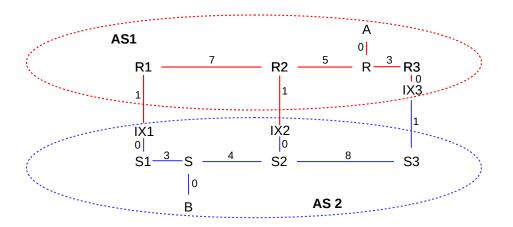
In the absence of the MED, AS1 will send traffic from A to B via the R3–IX3–S3 link, and AS2 will return the traffic via S1–IX1–R1. These are the links that are closest to R and S, respectively, representing AS1 and AS2's desire to hand off the outbound traffic as quickly as possible.
