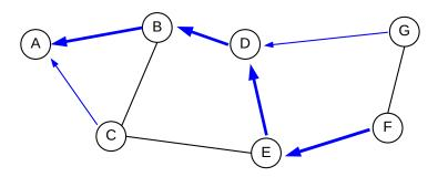
F now increments its own sequence number and creates a *RouteReply* message; F then sends it to A by following the highlighted (unicast) arrows above,  $F \rightarrow E \rightarrow D \rightarrow B \rightarrow A$ . As each node on the path processes the message, it creates (or updates) its route to the final destination, F; the return route to A had been created earlier when the node processed the corresponding *RouteRequest*.
