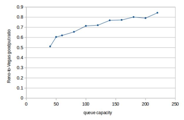
In this graph, TCP Vegas always gets more bandwidth than TCP Reno, though for large queue capacities Reno comes within 80%. The TCP Reno connection still faces bufferbloat problems, but the TCP Vegas connection is unaffected. (In the ns-2 simulator, SFQ's total queue capacity is set with, *eg*, Queue/SFQ set maxqueue\_ 100.)
