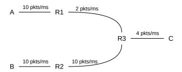
For a moment, assume R3 uses *priority* queuing, with the  $B \rightarrow C$  path given priority over  $A \rightarrow C$ . If B's flow to C is fixed at 3 packets/ms, then A's share of the R3–C link will be 1 packet/ms, and A's bottleneck will be at R3. However, if B's total flow rate drops to 1 packet/ms, then the R3–C link will have 3 packets/ms available, and the bottleneck for the A–C path will become the 2 packet/ms R1–R3 link.
