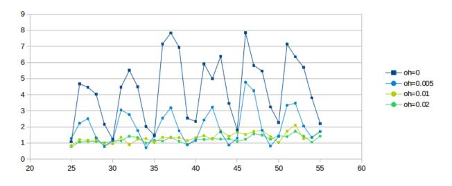
The dark-blue curve for overhead = 0 is wildly erratic due to phase effects; the light-blue curve for overhead = 0.005 has about half the oscillation. Even the light-green overhead = 0.01 curve exhibits some wiggling; it is not until overhead = 0.02 for the darker green curve that the graph really settles down. We conclude that the latter two values for overhead are quite effective at mitigating phase effects.
