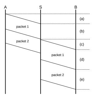
5.0. Now assume that the delays are the same as in exercise 4.0, except that the bandwidth delays are reversed: the A–S bandwidth delay is 157  $\mu$ sec and the S–B bandwidth delay is 103  $\mu$ sec. The propagation delays are unchanged. Draw the corresponding ladder diagram, and also the total time for two consecutive packets to be sent. (Hint: the total time should not change.)
