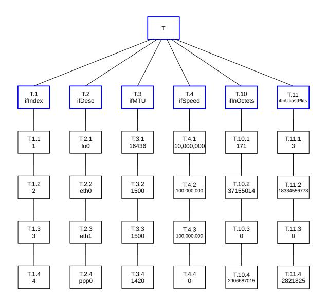
The diagram above emphasizes the arrangement into columns. The actual OID tree structure, however, is as in the diagram below; all the leaf nodes in one column above are actually sibling nodes.
