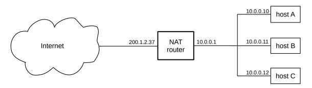
The remote machine responds, sending its responses to the NAT router's public IPv4 address. The NAT router remembers the connection, having stored the connection information in a special forwarding table, and forwards the data to the correct internal host, rewriting the destination-address field of the incoming packets.
