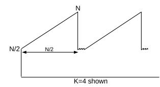
11.0. Suppose a TCP Reno tooth starts with cwnd = c, and contains N packets. Let w be the width of the tooth, in RTTs as usual. Show that  $w = (c^2 + 2N)^{1/2} - c$ . Hint: the maximum height of the tooth will be c+w, and so the average height will be c + w/2. Find an equation relating c, w and N, and solve for w using the quadratic formula.
