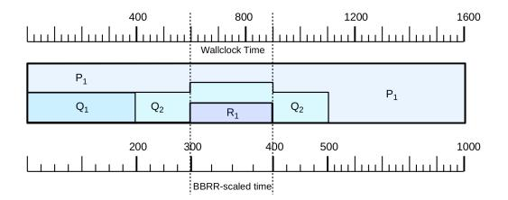
Under WFQ, the transmission order is  $Q_1$ ,  $Q_2$ ,  $P_1$ ,  $R_1$ , because when  $Q_2$  finishes at T=500,  $R_1$  has not yet arrived.
