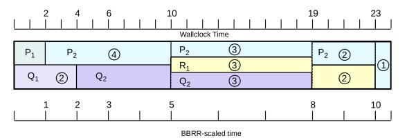
The circled numbers represent the size of the portion of the packet sent in the intervals separated by the dotted vertical lines; for each packet, these add up to the packet's total size.
