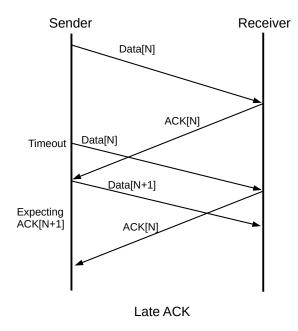
In this case we see that, after sending Data[N], receiving a delayed ACK[N] (rather than the expected ACK[N+1]) *must be considered a normal event*.
