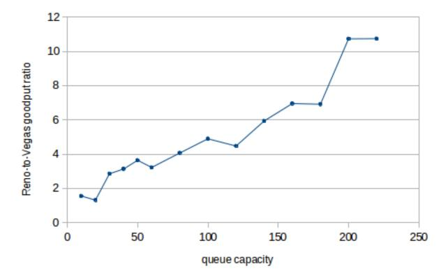
The vertical axis plots the Reno-to-Vegas goodput ratio; the horizontal axis represents the queue capacity. The performance of TCP Vegas falls off quite quickly as the queue size increases. One reason the larger  $\alpha$  may help is that this slightly increases the range in which TCP Vegas behaves like TCP Reno. (For a rather different outcome using fair queuing rather than FIFO queuing, see 23.6.1 Fair Queuing and Bufferbloat.)
