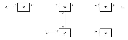
Fig. 14:: Five learning switches after three packet transmissions
