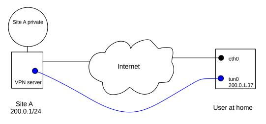
VPN: blue link represents *tunnel*. Actual connection is made via eth0 The tun0 interface is a virtual network interface with a Site-A address
