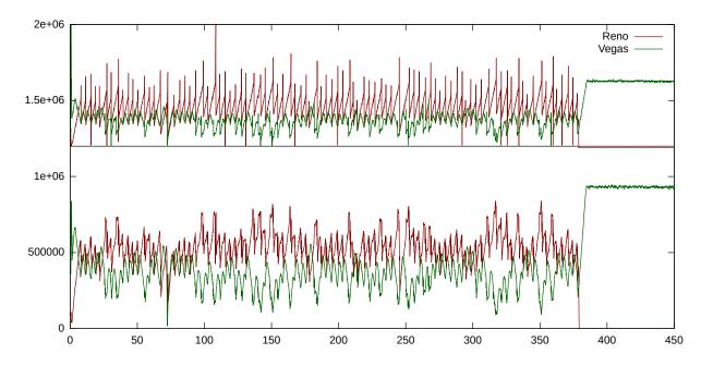
TCP Vegas is getting a smaller share of the bandwidth (overall about 40% to TCP Reno's 60%), but it is consistently holding its own. It turns out that TCP Vegas is greatly helped by the small queue size; if the queue size is doubled to 20, then Vegas gets a 17% share.
