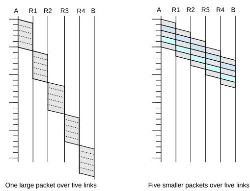
The point is that we can take advantage of parallelism: while the R4–B link above is handling packet 1,
