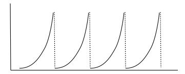
The number of packets sent in a tooth of width T RTTs, which is the reciprocal of the loss rate p, is now approximately  $T^3/3$  (this may be accepted on faith, or shown by integrating t<sup>2</sup> from 0 to T, or looking up the
