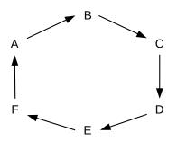
Packets will be transmitted in one direction (clockwise in the ring above). Stations in effect forward most packets around the ring, although they can also remove a packet. (It is perhaps more accurate to think of the forwarding as representing the default cable connectivity; *non*-forwarding represents the station's momentarily breaking that connectivity.)
