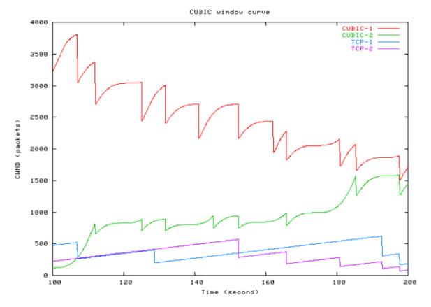
The diagram shows four connections, all with the same RTT. Two are TCP Cubic and two are TCP Reno. The red connection, cubic-1, was established and with a maximum cwnd of about 4000 packets when the other three connections started. Over the course of 200 seconds the two TCP Cubic connections reach a fair equilibrium; the two TCP Reno connections reach a reasonably fair equilibrium with one another, but it is much lower than that of the TCP Cubic connections.
