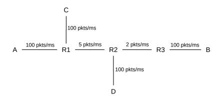
Initially, in the absence of C–D traffic, the A–B connection will send at a rate of 2 packets/ms (the R2–R3 bottleneck), and maintain a queue of four packets at R2. Because the RTT transit capacity is 10 packets, this will be achieved with a window size of 10+4 = 14.
