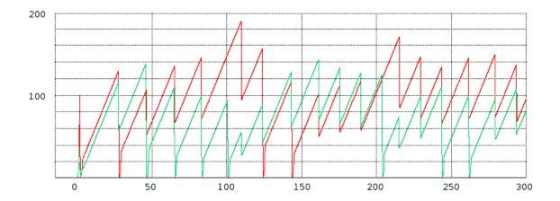
We start with the equal-RTTs graph, that is, delayB = 0. In this figure the teeth (loss events) are almost completely synchronized; the only unsynchronized loss events are the green flow's losses at T=100 and at about T=205. The two cwnd graphs, though, do not exactly move in lockstep. The red flow has three coarse timeouts (where cwnd drops to 0), at about T=30, T=125 and T=145; the green flow has seven coarse timeouts.
