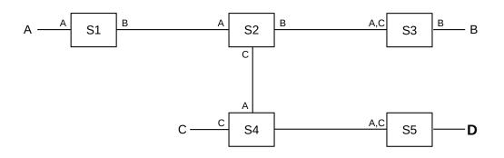
Which switches will see this  $D \rightarrow B$  packet, and thus learn about D? Of these switches, which do *not* already know where B is and will use fallback-to-flooding?
