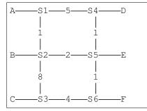
The links between switches are labeled with **weights**, which are used by some routing applications. The weights represent the cost of using that link. You are to find the path through S1-S6 with lowest total cost (that is, with smallest sum of weights), for each of the following transmissions. For example, the lowest-cost path from A to E is A-S1-S2-S5-E, for a total cost of 1+2=3; the alternative path A-S1-S4-S5-E has total cost 5+1=6.
