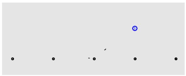
Above is one frame from the animation, with the mover node is almost (but not quite) directly over rownode (3), and so is close to losing contact with rownode (2). Two CBR packets can be seen *en route*; one has almost reached rownode (2) and one is about a third of the way from rownode (2) up to the blue mover node. The packets are not shown to scale; see exercise 17.
