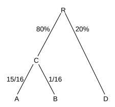
When A is idle, B gets 4 times D's bandwidth When A is active, B gets 1/4 D's bandwidth
