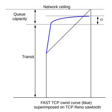
The diagram above illustrates a FAST TCP graph of cwnd versus time, in blue; it is superimposed over one sawtooth of TCP Reno with the same network ceiling. Note that cwnd rises rapidly when it is below the path transit capacity, and then levels off sharply.
