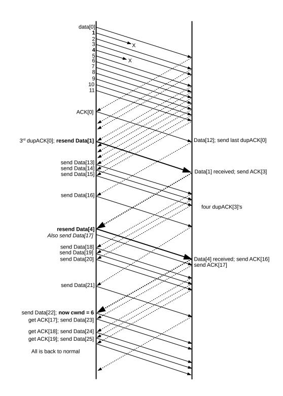
When the receiver's first ACK[3] arrives at the sender, NewReno infers that Data[4] was lost and resends it; this is the second heavy data line. No dupACK[3]'s need arrive; as mentioned above, the sender can infer from the single ACK[3] that Data[4] is lost. The sender also responds as if another dupACK[0] had arrived, and sends Data[17].
