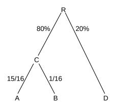
When A is idle, B gets 4 times D's bandwidth When A is active, B gets 1/4 D's bandwidth
