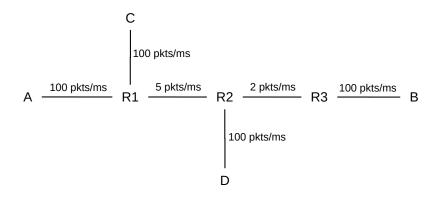
Let us suppose the A–B link is idle, and the C $\longrightarrow$ D connection begins sending with a window size chosen so as to create a queue of 30 of C's packets at R1 (if propagation delays are such that two packets can be in transit each direction, we would achieve this with winsize=34).
