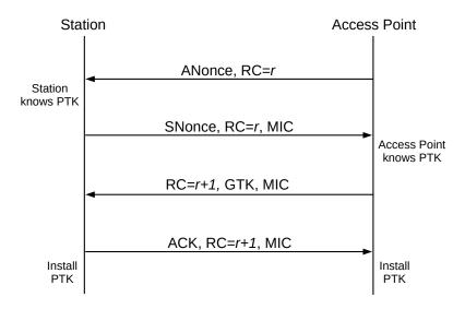
Fig. 27:: Four-way WPA2 handshake; RC represent the replay counter
