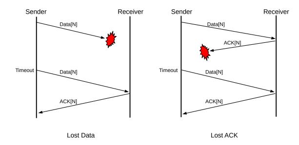
The right half of the diagram, by comparison, illustrates the case of a lost ACK. The receiver has received a *duplicate* Data[N]. We have assumed here that the receiver has implemented a **retransmit-on-duplicate** strategy, and so its response upon receipt of the duplicate Data[N] is to retransmit ACK[N].
