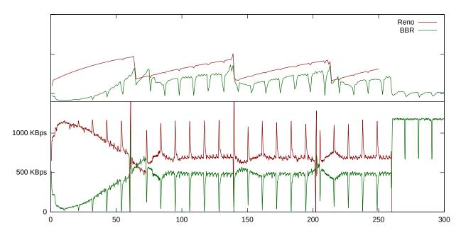
For the first ten seconds, TCP Reno does indeed run away with all the bandwidth. But after the first PROBE\_RTT event TCP BBR begins to catch up, and the two tie at around T=60 seconds. After that Reno mostly stays a little ahead of TCP BBR, typically with about 58% of the bandwidth versus BBR's 42%, but the point here is that, even in circumstances favorable to Reno, BBR does not collapse.
