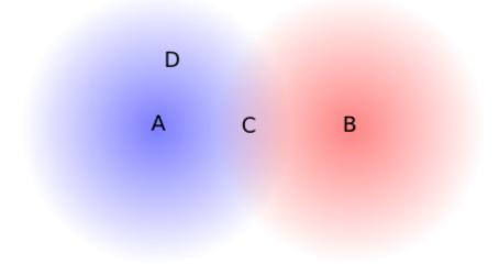
Fig. 20:: If A and B transmit simultaneously, there is a collision at C, reachable by both, but not at D
