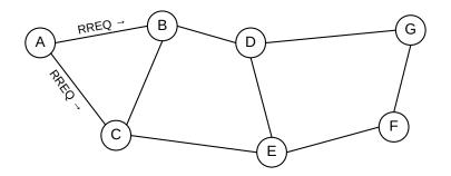
The *RouteRequest* is sent initially to A's direct neighbors, B and C in the diagram above, using UDP. We will assume for the moment that the *RouteRequest* reaches all the way to F before a *RouteReply* is generated.
