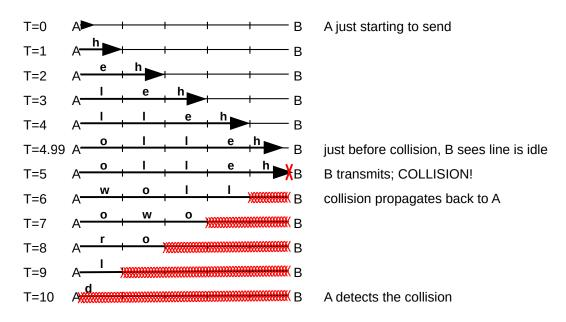
Fig. 10:: Ethernet collision, showing one full RTT before collision detectability
