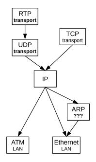
Fig. 7:: A protocol graph TCP and UDP/RTP are above IP, and ATM and Ethernet are below
