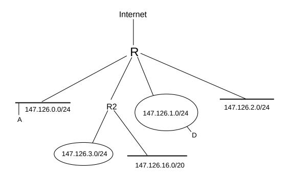
What we want is for the internal routing to be based on the extended network prefixes shown, while externally continuing to use only the single routing entry for 147.126.0.0/16.
