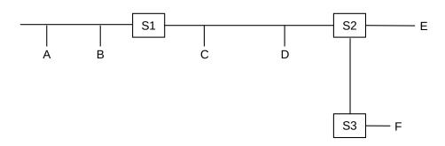
Fig. 13:: Ethernet with switches S1, S2 and S3
