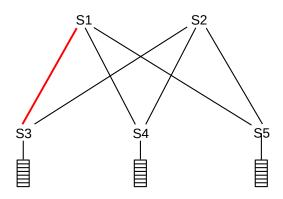
One goal here is to ensure that, if the S1–S3 link fails, data is routed over the two paths S1–S4-S2–S3 and S1–S5–S2–S3. To this end, we begin by making each of S1 through S5 its own AS. Later, the set of S1 through S5 will be treated as a single AS, using **AS confederation** (**RFC 5065**). Because S1 through S5 do not export their individual AS numbers outside the confederation, the same AS numbers can be reused over and over.
