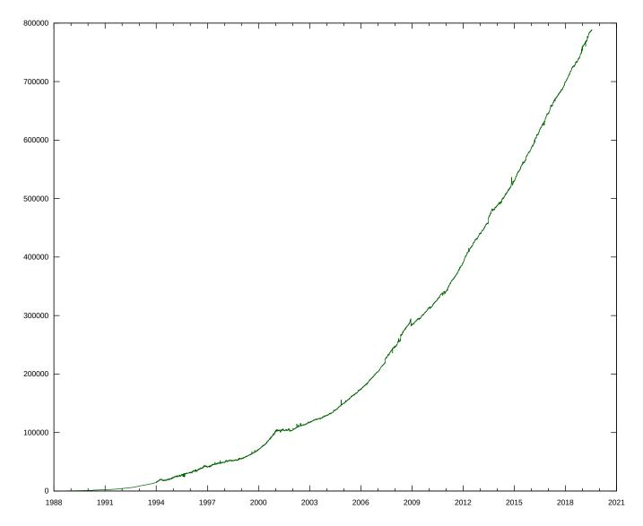
The time range is from 1994 to July 2019; at the end, there are 788 thousand IP prefixes from (not shown in the graph) around 65 thousand Autonomous Systems. The graph is flat from 2001 to 2002, reflecting the aftereffects of the so-called dot-com bubble. Overall the increase with time is roughly quadratic, but in the last decade has been closer to linear.
