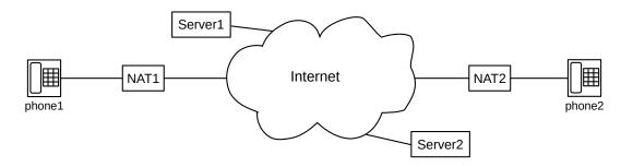
For phone1 to call phone2, phone1 first contacts Server1, which then contacts Server2. So far, all is well. The final step is for Server2 to contact phone2, which, however, cannot be done normally as NAT2 allows
