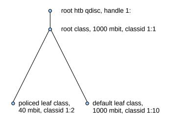
To create the htb hierarchy we will first create the root qdisc and associated root *class*. We need the raw interface rate, here taken to be 1000mbit. Class identifiers are of the form *major:minor*, where *major* is the integer root "handle" and *minor* is another integer. (We do not absolutely need to create a root class, but only children with a common parent *class* can share bandwidth.)
