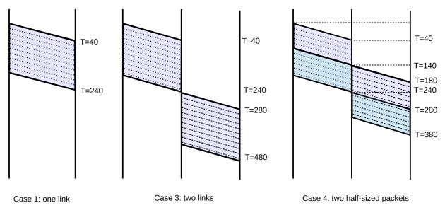
Bandwidth delay 200  $\mu sec,$  per-link propagation delay 40  $\mu sec$
