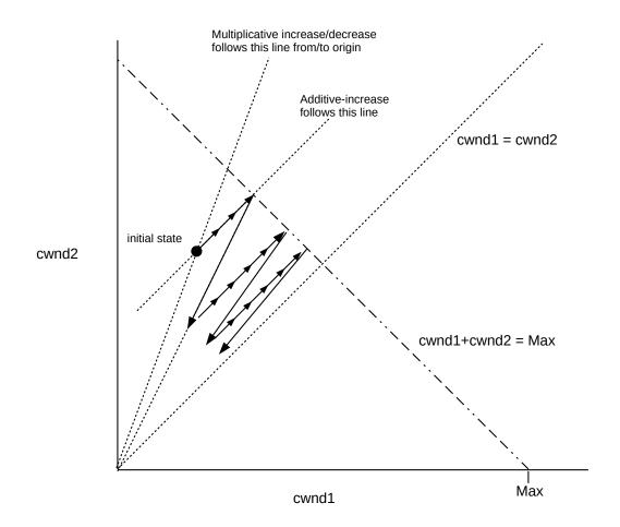
Beginning at the initial state, additive increase moves the state at a  $45^{\circ}$  angle up to the line x+y=Max, in small increments denoted by the small arrowheads. At this point a loss would occur, and the state jumps back halfway *towards the origin*. The state then moves at  $45^{\circ}$  incrementally back to the line x+y=Max, and continues to zigzag slowly towards the equal-shares line y=x.
