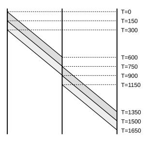
The long propagation delay means that A finishes all transmissions before S begins receiving anything, and S finishes all transmissions before B begins receiving anything. With a smaller propagation delay, these A/S/B events are likely to overlap.
