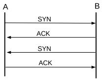
Possible four-way handshake Less secure than three-way version
