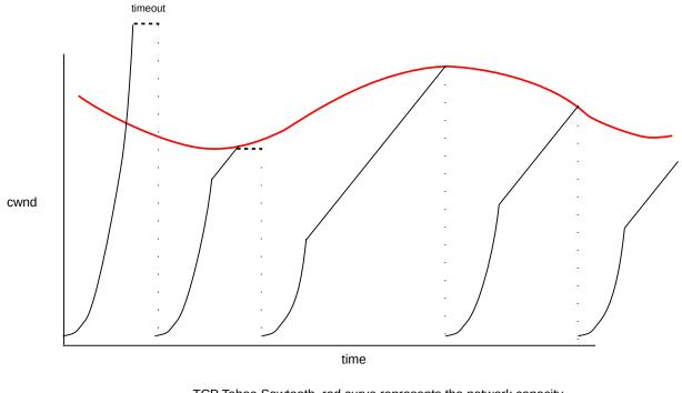
TCP Tahoe Sawtooth, red curve represents the network capacity Slow Start is used after each packet loss until ssthresh is reached
