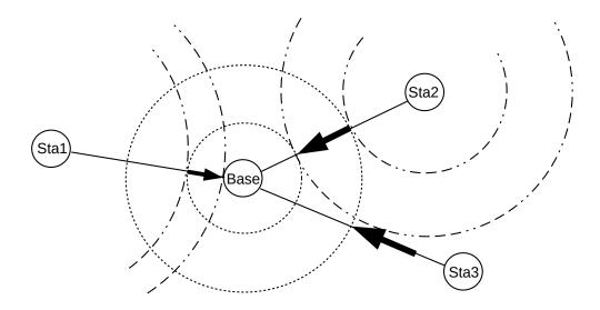
Fig. 29:: Three packets in transit from stations Sta1, Sta2 and Sta3. The packets propagate outwards from the stations at the speed of light, like ripples, spatially confined between two concentric dot-dash circles (circles around Sta3 are not shown). The packet portion along the straight line from the station to the Base is represented as a heavy arrow. The three packets will arrive at Base sequentially and without overlap.
