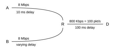
Broadly speaking, the simulations here will demonstrate that the longer-delay B–D connection receives less bandwidth than the A–D connection, but not quite so much less as was predicted in 20.3 *TCP Reno Fairness with Synchronized Losses*. The synchronized-loss hypothesis increasingly fails as the B–R delay increases, in that the B–D connection begins to escape some of the packet-loss events experienced by the A–D connection.
