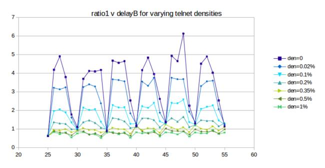
As we hoped, the oscillation does indeed substantially flatten out as the telnet density increases from 0 (dark blue) to 1% (bright green); the mean deviation falls from 1.36 to 0.084. So far the use of telnet is very promising.
