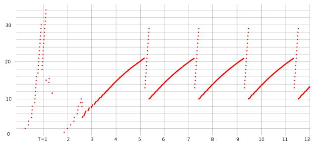
When we run the script and plot the cwnd trace data (here for about 12 seconds), we get the following:
