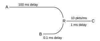
In the diagram above, the A–C connection wants its cwnd to be about 200 ms  $\times$  10 packets/ms = 2,000 packets; it is competing for the R–C link with the B–D connection which is happy with a cwnd of 22. If R's queue capacity is also about 20, then with most of the bandwidth the B–C connection will experience a loss about every 20 RTTs, which is to say every 22 ms. If the A–C link shares even a modest fraction of those losses, it is indeed in trouble.
