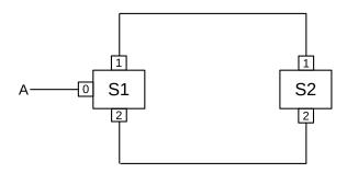
Suppose A attempts to send a packet to destination B, which is unknown. S1 will therefore flood the packet out interfaces 1 and 2. What happens then? How long will A's packet circulate?
