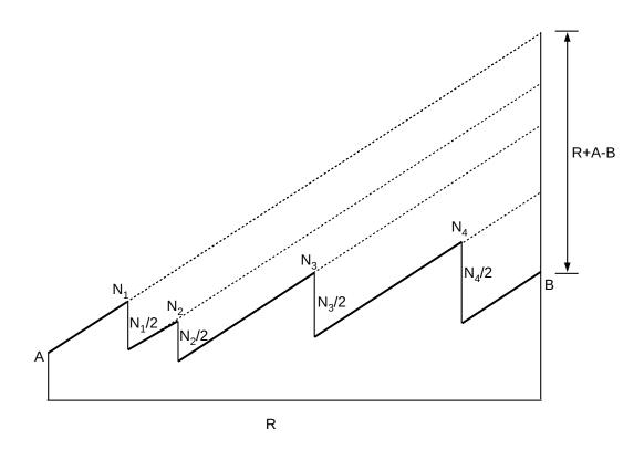
8.0. Suppose the bandwidth×delay product for a network path is 1000 packets. The only traffic on the path is from a single TCP Reno connection. For each of the following cases, find the average cwnd and the approximate number of packets between losses (the reciprocal of the loss rate). Your answers, collectively, should reflect the formula in 21.2 TCP Reno loss rate versus cwnd.
