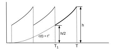
Note that as the teeth here become higher, they become proportionately narrower. Hint: show  $T_1 = (0.5)^{0.5} \times T$ , and then eliminate  $T_1$  from the above equations.
