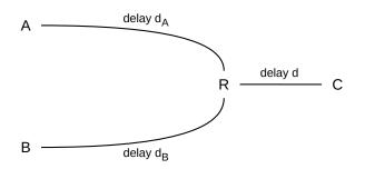
The network layout here, with the shared R–C link as the bottleneck, is sometimes known as the **singlebell** topology. A perhaps-more-common alternative is the **dumbbell** topology of 20.3 TCP Reno Fairness with Synchronized Losses, though the two are equivalent for our purposes.
