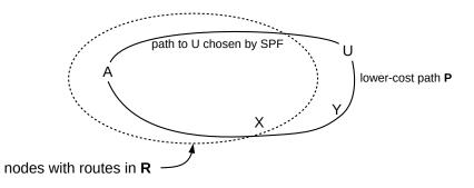
At some strictly earlier stage in the algorithm, we must have added a route to node X, as the route to X is in **R**. In the following stage, we would have included the prefix  $\langle A, ..., X, Y \rangle$  of **P** in Tentative. This path to Y has cost  $\leq c$ . This route must still be in **T** at the point we chose U as **current**, as there is no route to Y in **R**, but this means we should instead have chosen Y as **current**, contradicting the choice of U.
