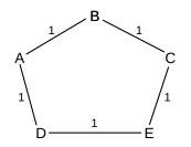
Now suppose the D–E link fails, and so D updates its entry for E to  $\langle E, -, \infty \rangle$ .
