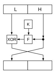
One round here scrambles only half the block, but the other half gets scrambled in the next round (sometimes the operation above is called a half-round for that reason). The total number of rounds is typically somewhere between 10 and 50. Much of the art of designing high-quality block ciphers is to come up with round functions that result in overall very fast execution, without introducing vulnerabilities. The more rounds, the slower.
