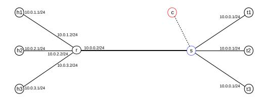
The servers all get the *same* IPv4 address, 10.0.0.1. This would normally lead to chaos, but the servers are not allowed to talk to one another, and the controller ensures that the servers are not even aware of one another. In particular, the controller makes sure that the servers never all simultaneously reply to an ARP "who-has 10.0.0.1" query from r.
