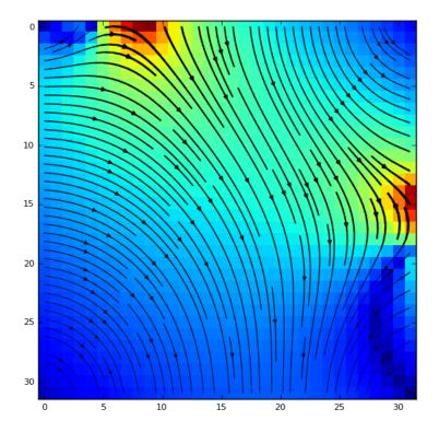
If the fluid is flowing along the top then down the right-hand edge, rather than through the middle of the cavity, then this is an indication that the Jacobi algorithm has not yet converged. Convergence requires more iterations on larger problem sizes.
