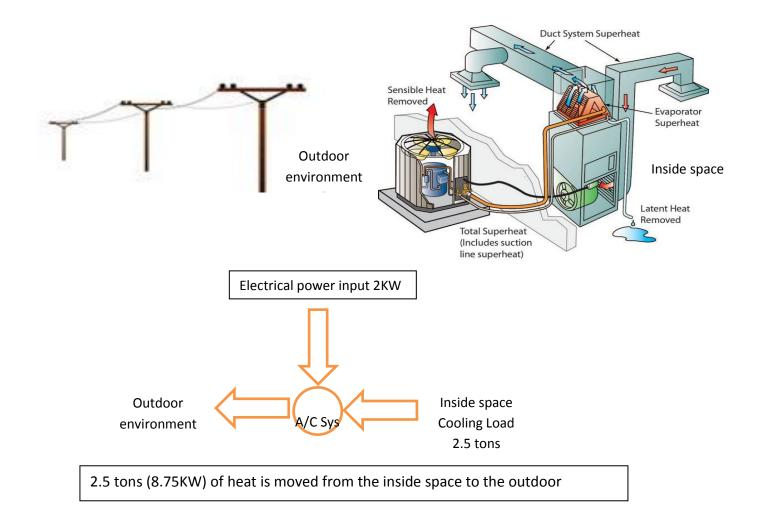
Consider the figure above and example, the cooling load is calculated to be approx. 2.5 tons. The A/C system selected to cool this space is specified as a 2.5-ton system with 230VAC input and R.L. (Running Load) of 9 amps. Most manufactures size residential A/C systems in 0.5 ton increments so this works out very well at 2.5 tons.
