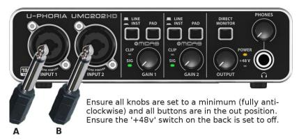
The gain controls on the front of the UMC20xHD can be used to give a little extra level if required but ensure the level meters in the Graff software do not hit the top otherwise distortion will be introduced.
