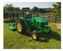
**Mow pastures, brush, and roadsides.** Rotary cutters, powered by the tractor's PTO, handle tough cutting and mowing jobs, and are perfect for pastures or other big, open spaces. Most rotary cutters are available in several sizes and duty levels.
