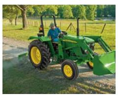
**Grade and blade.** Hitch up to a rear blade, and you can level paths or gravel driveways.
