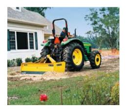
**Dirt or materials work.** If it needs to be smooth as glass, go over it with a box blade, land plane, or other leveling implement to re-grade or fill potholes.
