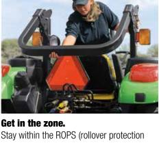
Stay within the ROPS (rollover protection structure) zone. This U-shaped bar over the seat protects you in case of a rollover.
