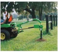
**Save your back.** A posthole digger is a must-have if you're putting up a fence. Powered by the PTO. the auger digs perfect postholes, every time.
