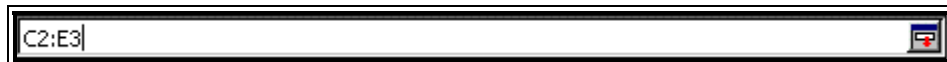
Figure 48: Selecting the cell references whose values will be the inputs into the function
