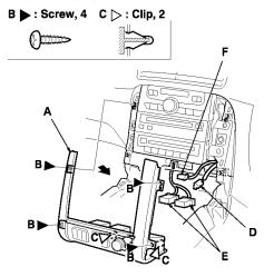
4. Detach the clips and release the hooks (A), then remove the driver's console side trim (B) and passenger's console side trim (C).
