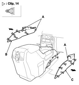
5. Starting at the top, gently pull out the console rear trim (A) to detach the clips (B), then pull out the trim to detach the remaining clips (C), and disconnect the rear heater-A/C passenger's control panel-unit connectors (D) and console accessory power socket connector (E). If equipped with rear entertainment system, disconnect the rear entertainment system jack connector (F).
