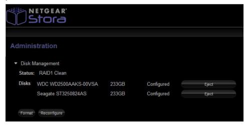
You can maximize data protection by adding a second backup disk to your RAID1 configuration. When you add a second disk, the data stored on the first disk is copied to the second disk as a mirrored backup and protects your data against disk failure and loss.
