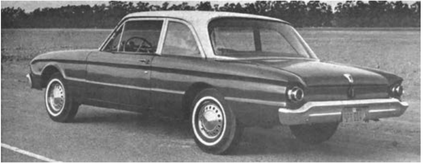
The missing three inch section is not as obvious as one might expect; the tail lights and arched rear wheel cutouts being giveaways.
