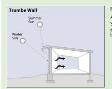
Figure 1: A trombe wall. Source: <u>http://energy.gov/</u> energysaver/passive-solarhome-design
