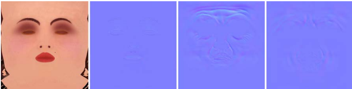
Figure 2. Ruby's face textures (left to right): albedo map, tangent space normal map, tangent space wrinkle map 1 for stretched face, and tangent space wrinkle map 2 for compressed face.
