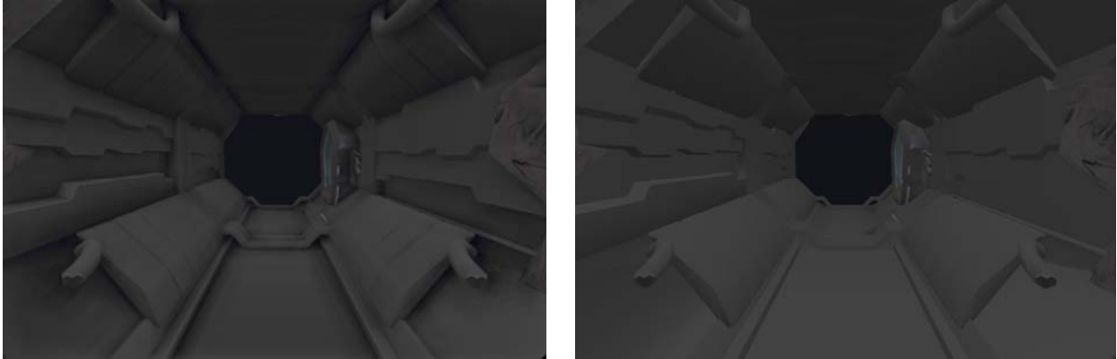
Figure 17. Sample scene B with special material setup to visualize SSAO (left: with SSAO, right: without SSAO)
