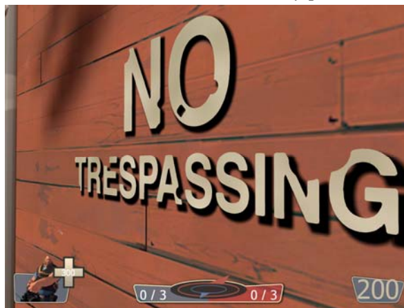
Figure 7. Soft drop-shadow added by the pixel shader. The direction, size, opacity, and color of the shadow are dynamically controllable.
