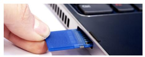
**NOTE:** Ensure the SD card is unlocked (not write-protected). The lock slider on the side of the SD card should be in the up position.
