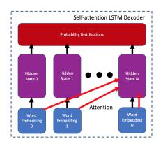
Figure 3: LSTM decoder with self-attention
