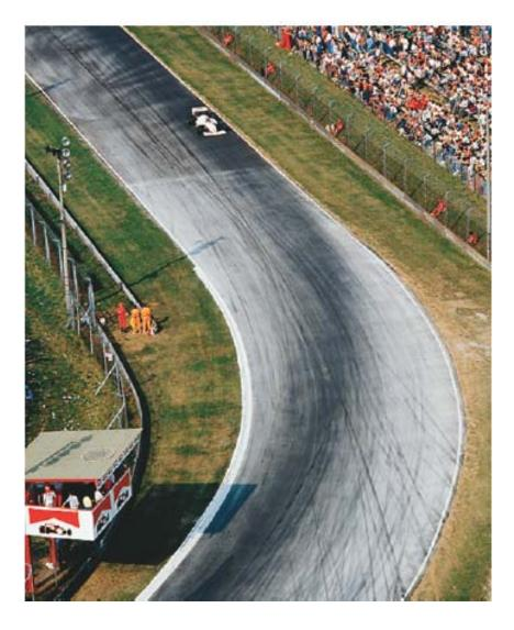
If the frictional force is insufficient, the car will tend to move more nearly in a straight line, as the skid marks show.
