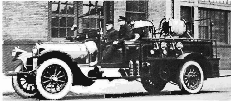
PIERCE ARROW chassis with a chemical engine, 1924, built by H. E. Penney after he left the Nott Fire Engine Company
