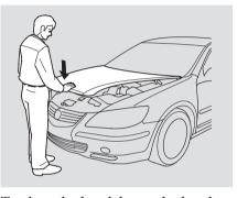
To close the hood, lower the hood to about a foot (30 cm) above the fender, then firmly press down on the front edge of the hood. Make sure it is securely latched.
