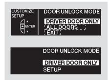
You can select whether the driver's door unlocks or all the doors unlock when you unlock the doors by grabbing the driver's door handle while carrying the remote. Select the desired mode by pressing the ▲ or ▼ button, and enter your selection by pressing the SEL/RESET button.
