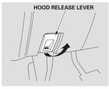
1. Park the vehicle, and set the parking brake. Pull the hood release lever located under the lower left corner of the dashboard. The hood will pop up slightly.
