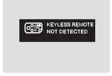
When you are pressing the ignition switch, or when the ignition switch is in the ON (II) position, the beeper sounds if you take the remote out of the vehicle and close the door
