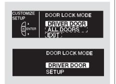
If you unlock the doors by pressing the button on the remote, you can select whether the driver's door unlocks or all the doors unlock. Select the desired mode by pressing the ▲ or ▼ button, and enter your selection by pressing the SEL/RESET button.
