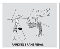
To apply the parking brake, push the parking brake pedal down with your foot. To release the parking brake, push on the pedal again. The parking brake indicator on the instrument panel should go out when the parking brake is fully released with the engine running (see page 61).
