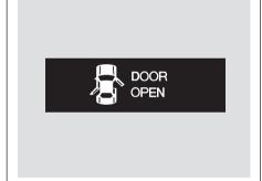
When one or more doors are not tightly closed, the "DOOR OPEN" indicator will stay on.
