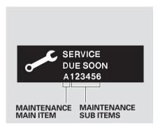
When the remaining engine oil life is 15 to 6 percent, the multi-information display shows a "SERVICE DUE SOON" message along with the maintenance schedule code indicating the main and sub items required at the time of the oil change. Refer to page 299 and 300 for a complete list of the maintenance main items and sub items.
