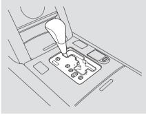
To shift from any position, press firmly on the brake pedal and slide the lever along the guide on the console. You cannot shift out of Park when the ignition switch is in the LOCK (0) or ACCESSORY (I) position.
