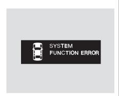
If there is a system error with the TPMS, the multi-information display shows a "SYSTEM FUNCTION ERROR" message (see page 72 ), and the tire pressure readings will not be displayed. You will also see a "CHECK TPMS SYSTEM" message on the multi-information display (see page 280 ).
