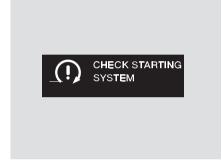
If there is a problem with the starting system, you will see a "CHECK STARTING SYSTEM" message on the multi-information display when the ignition switch is turned to ON (II). You will also see this message when the auto control mode of the starting system has a problem.
