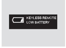
The batteries in the remote normally lasts about 2 years. To ensure maximum battery life, do not store the remote close to electrical devices such as computers or TVs. When the multi-information display shows "KEYLESS REMOTE LOW BATTERY," replace the batteries as soon as possible (see page 135).
