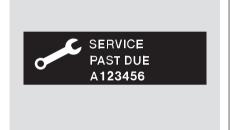
If the indicated maintenance service is not done and the remaining engine oil life reaches 0 percent, the multi-information display will show the message "SERVICE PAST DUE" and the maintenance item code. This message is displayed when the total mileage after reaching 0 percent engine oil life is less than 10 miles (for U.S. models)/10 km (for Canadian models).
