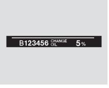
Press the SEL/RESET button on the steering wheel repeatedly to select the engine oil life minder, the message "CHANGE OIL" along with the percentage "5%," and the maintenance item code are displayed on the lower part of the multi-information display when the calculated engine oil life is 1-5 percent (see page 291).
