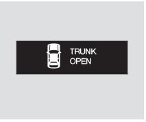
When the trunk is not tightly closed, the "TRUNK OPEN" indicator will stay on.
