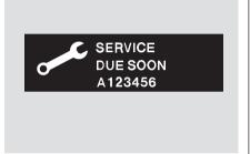
When the engine oil life reaches 15 percent, the display shows "SERVICE DUE SOON" and the code for the maintenance items to be performed.
