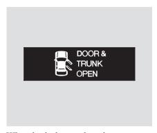
When both the trunk and one or more doors are not tightly closed, the "DOOR & TRUNK OPEN" indicator will stay on.
