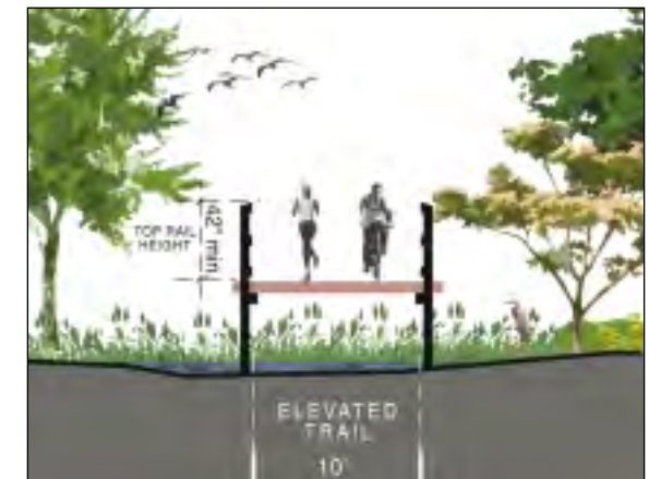
Elevated Trail Example of raised boardwalk section over wetlands or natural area, to be incorporated as part of tributary crossings or in places where views over wetlands are desired.
