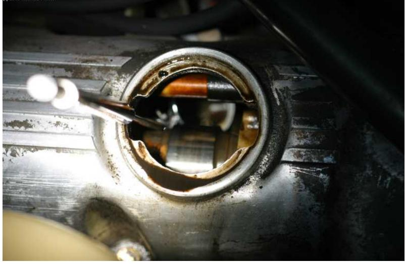
Angle it to where you can see the chain (it's all the way on the front of the engine):
