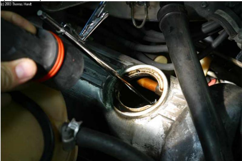
Mercedes-Benz - Timing Chain Inspection 380 V8 Engines
