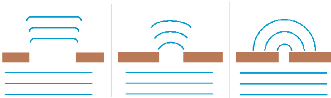
Fig 3.5.1 Waveforms after passing a gap. Note how the width of the gap influences the shape of the wavefronts. After passing through the gap, the wavelength is not changed.
