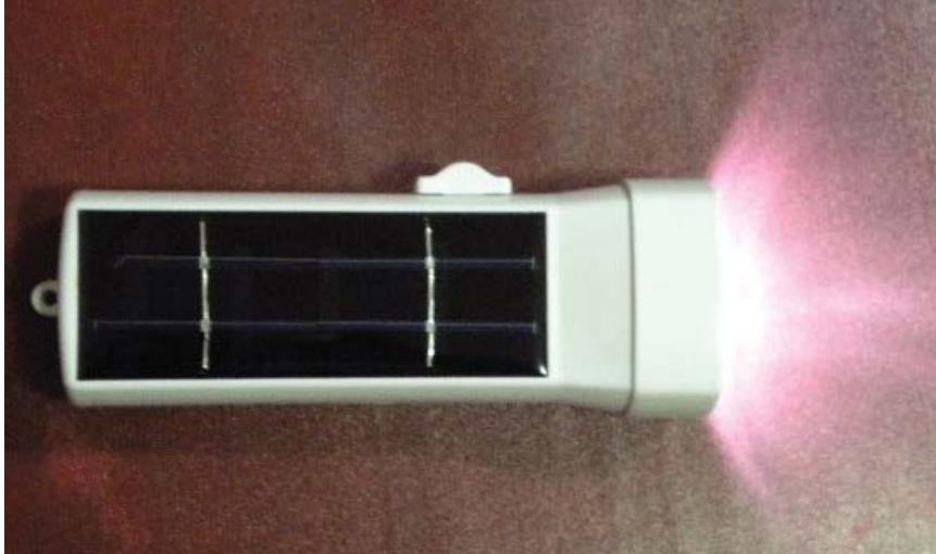
Fig 5.3.1 Torch powered by solar cells
