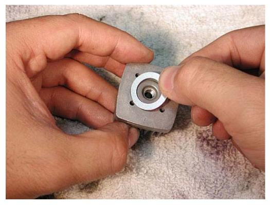
Carefully install the head as shown below, so the head shim doesn't fall off the head.
