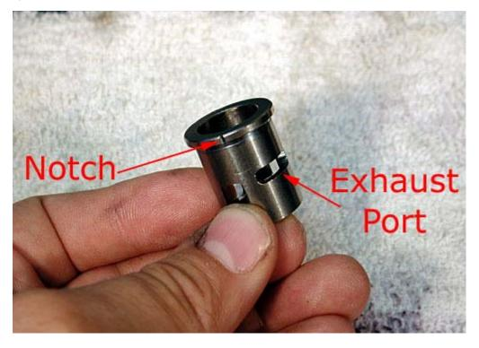
lin the picture below the notch in the sleeve faces directly away from the camera. Note that the large hole in the piston must NOT face the exhaust port. Some engines do not use pistons with a hole, however remember this example engine is the 15FE - this is the type of piston it must use.
