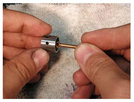
Get the new piston, the wrist pin and connecting rod and reverse the procedure you just did to remove the wrist pin. Put the thin end of the con rod into the piston.
