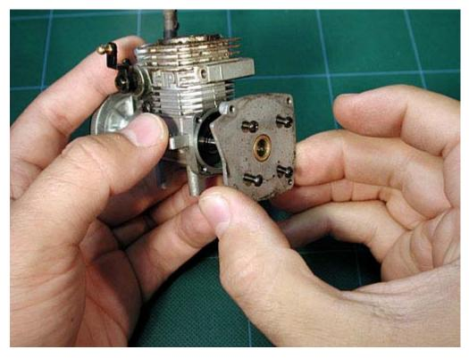
You will now have the interior of the engine exposed. Pullstarter-equipped engines will
