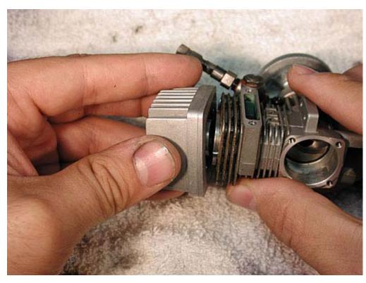
Remember how the head was positioned on the engine.
