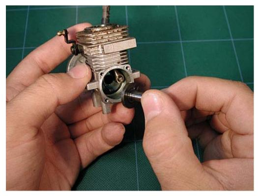
Use a pair of pliers to loosen the engine sleeve from the engine case.
