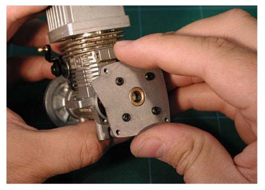
Install the pullstarter and tighten the screws. Use the "star" technique - it isn't absolutely necessary for the pullstarter, but get in the habit of using this technique on all parts on your engines.
