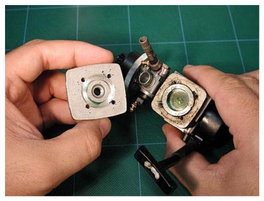
Use the right screwdriver to take off the pullstarter. For the 15FE, a #2 screwdriver is needed for this. If your engine does not have a pullstarter, take off the backplate and skip the next couple of steps.
