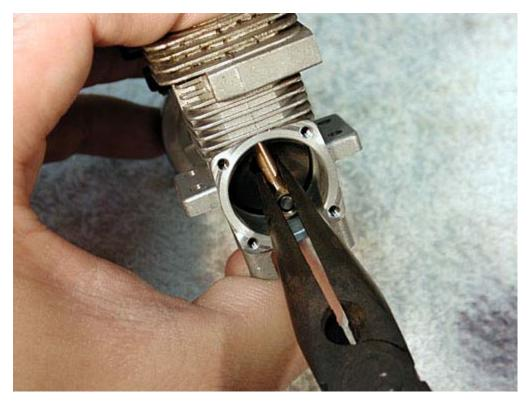
If the piston comes out of the bottom of the sleeve while you're positioning the con rod, don't worry. Use a hobby knife to gently push the piston into the sleeve again.
