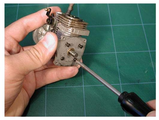
Remove the pullstarter plate and put it next to the engine head and pullstarter.
