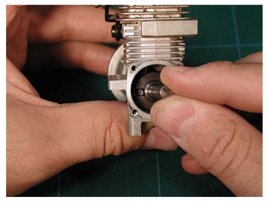
Install the pullstarter plate and tighten the screws. Use the "star" technique - it isn't absolutely necessary for the pullstarter, but get in the habit of using this technique on all parts on your engines. Because the head shim package for the 15FE includes a pullstart gasket, you can replace the gasket on the pullstarter plate if you wish.
