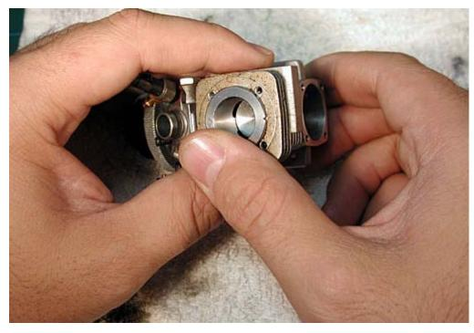
Set the engine case aside. Get the engine head and pull out the head shim with a hobby knife.
