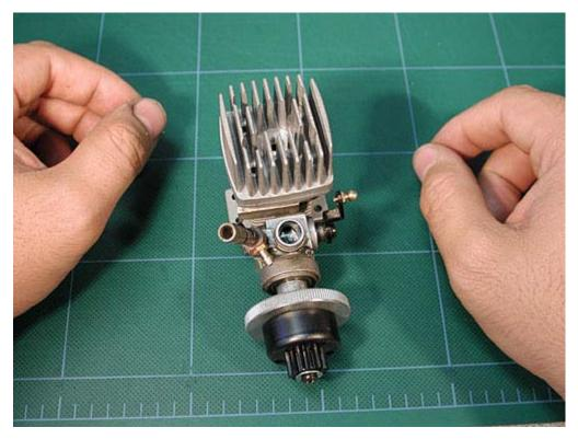
Install the head screws to hold the head in place. When you start to feel resistance, STOP turning the screwdriver.
