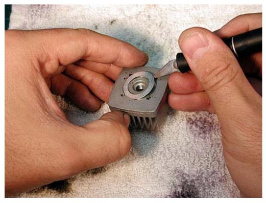
Use Nitro Car Cleaner to spray away any dirt from the screw holes and bottom of the head.
