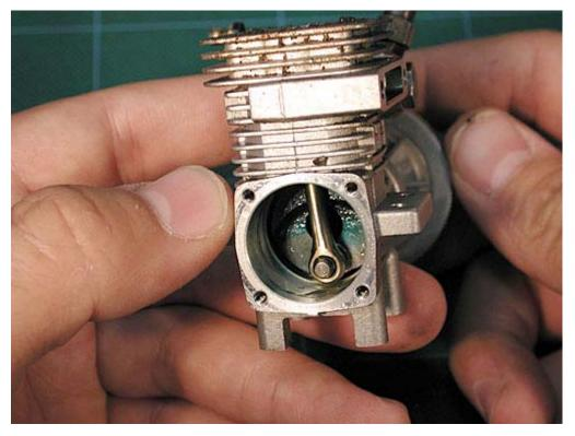
Use a pair of needlenose pliers to pull the bottom of the connecting rod off the cam. If you
