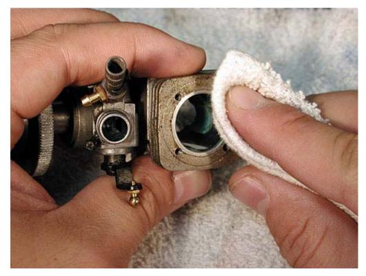
Now we will start the process of installing the new piston and sleeve into the engine case. HPI engines have a notch in the top of the sleeve. This notch must face to the rear of the engine (towards the pullstarter or back plate). Find this notch and insert the piston through the bottom of the sleeve.
