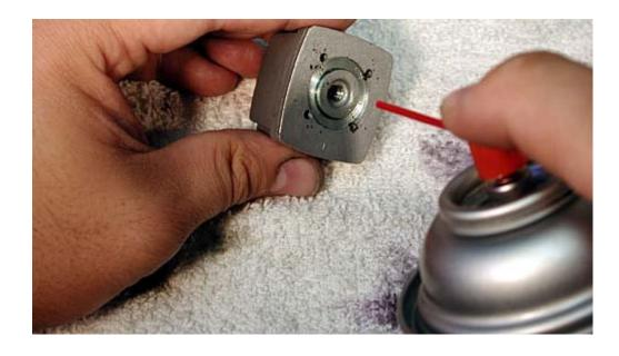
The bottom of the heat sink head should be pretty clean before installation.
