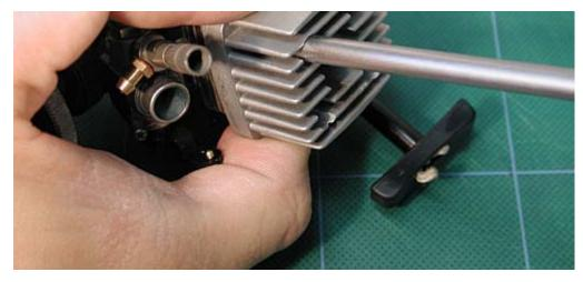
Now that you have the heat sink head off, set it aside also. Remember the way the fins faced so later on you won't have to reposition the head after you install it in your car or truck.
